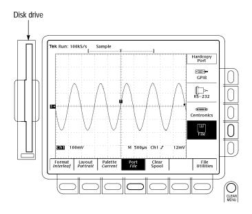
4 Press **HARDCOPY** anytime to save a copy of the current screen to a unique file in the oscilloscope file system.
