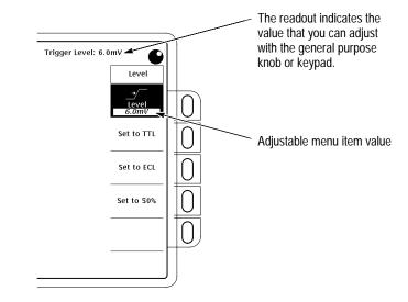
4 Adjust menu item values using the general purpose knob or by entering numbers on the keypad.
