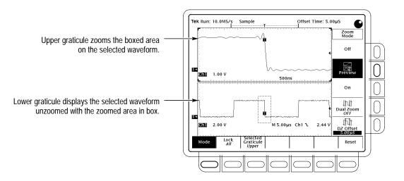
**3** Use the **Selected Graticule** menu to select the upper or lower waveform. Use the vertical and horizontal knobs to adjust the waveform in the graticule you select.
