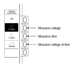
4 Move the cursor with the general purpose knob. Press SELECT to switch between the cursors. Press SHIFT to speed up/slow down the cursor movement.
